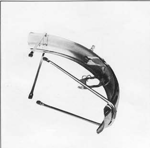
STEP 37 — Assemble front fender braces as shown.
