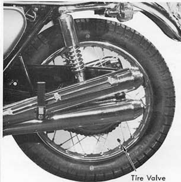
STEP 80 — Check tire pressure. Front: 28 PSI Rear: 30 PSI
