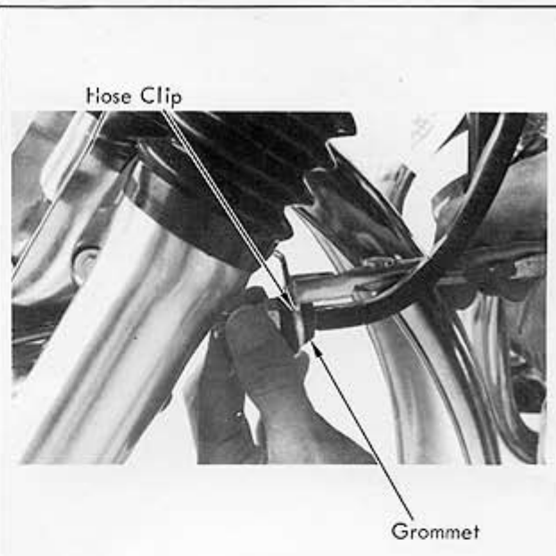
STEP 42 — Press brake hose grommet into hose clip attached on fender bracket. Squeeze clip with pliers to retain grommet.
