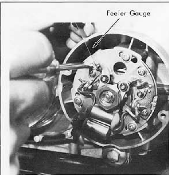
STEP 71 — Check point gap. Adjust points, if necessary, as described in the owner's manual or shop manual. Point gap: 0.3 - 0.4 mm (0.012 - 0.016 in.)
