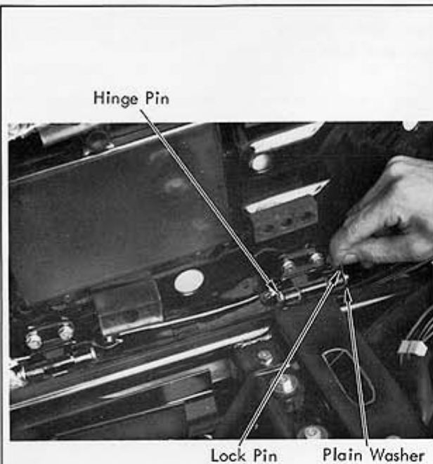
STEP 77 — Install seat using two seat hinge pins, plain washers, and lock pins. Insert hinge pins so heads of pins are towards each other.
