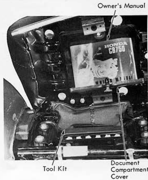
STEP 78 — Insert tool kit in tray next to battery. Insert owner's manual in document compartment.
