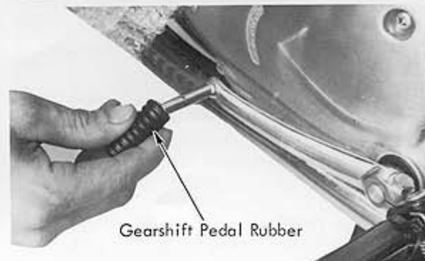
STEP 57 — Install kick starter pedal and gearshift pedal rubbers.
