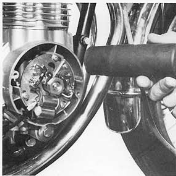
STEP 73 — Using a stroboscopic timing light, check ignition timing at idle and at full advance. Time cylinders 1 and 4, then time cylinders 2 and 3. Adjust timing, if necessary, as described in owner's manual or shop manual. Reinstall cover.
