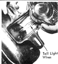
STEP 34 - Connect the tail light wires.
