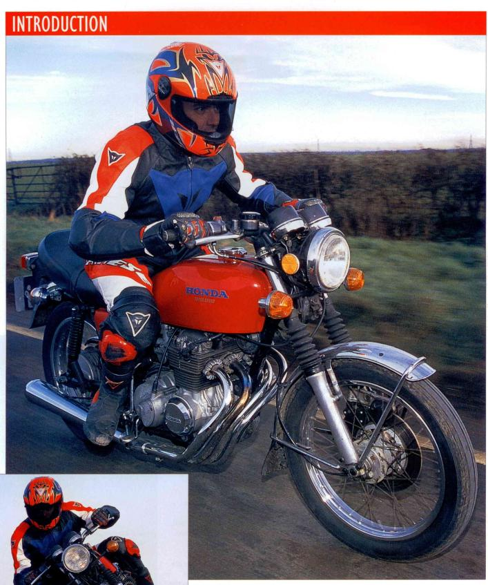
ONDA'S innovative lightweight multi created a huge stir when unveiled in 1974. Based on the existing CB350/4 (which was never officially imported into the UK, unlike the popular CB500 which shared similar styling), it used substantially the same engine but had a bore increase from 47 to 51mm.
