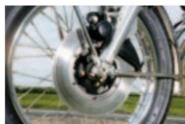
Sliding piston caliper is prone to wintertime corrosion
