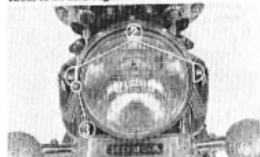
(2) Headlight mounting bolts (3) Beam adjusting screw
